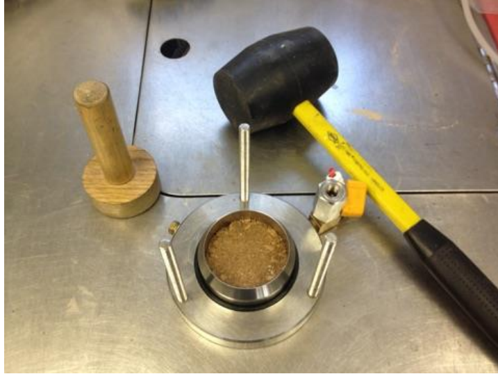
Figure 25. Setup for compaction of backfill material in oedometer
