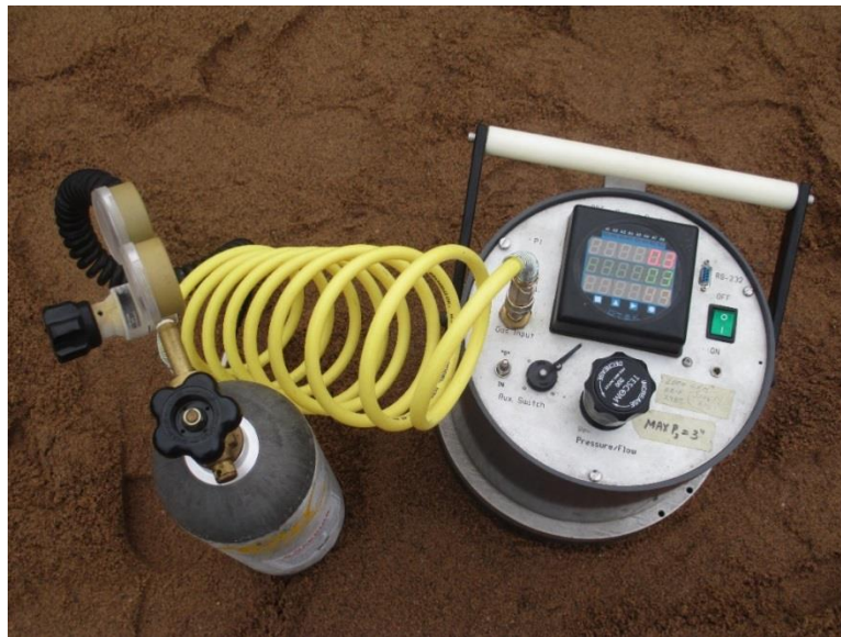
Figure 36. Air permeability testing at Slovak Valley Creek Bridge
