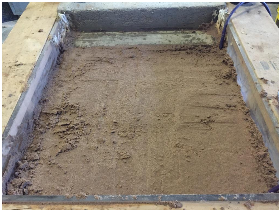
Figure 75. Top of backfill after testing Schwartz road backfill material with geocomposite vertical drain (top view)
