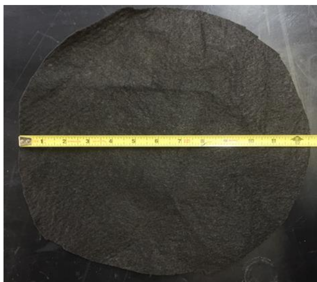
Figure 24. Geosynthetic fabric used in permeability testing
