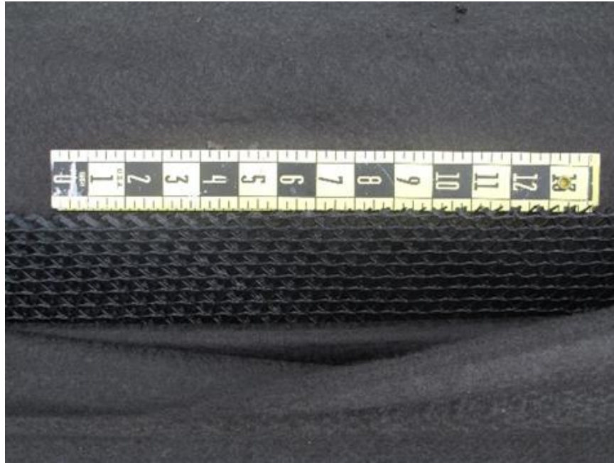
Figure 72. Roadrain T5 geocomposite drain
